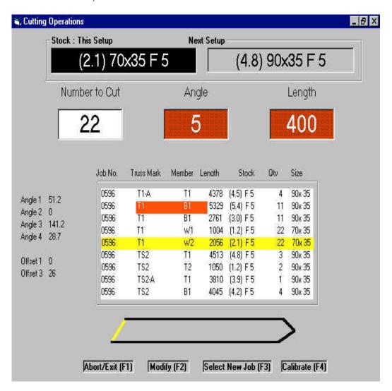
**Stock:** Which timber stock is required for the current member and the next member in the list The background colour changes according to the grade of timber required.
