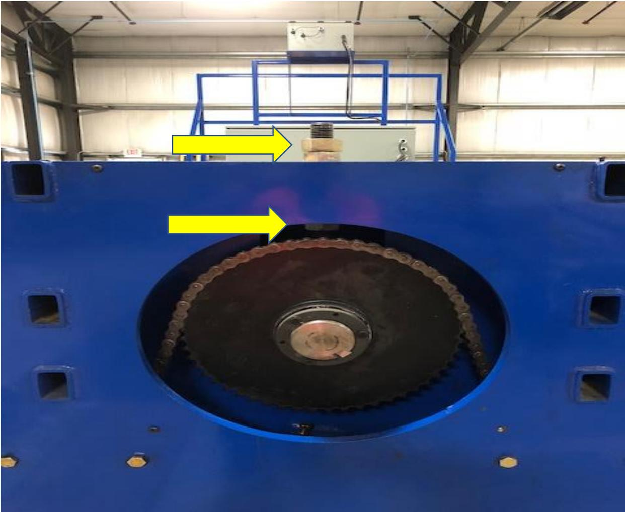
Location of Roll Height Adjustment Jam Nut Location
