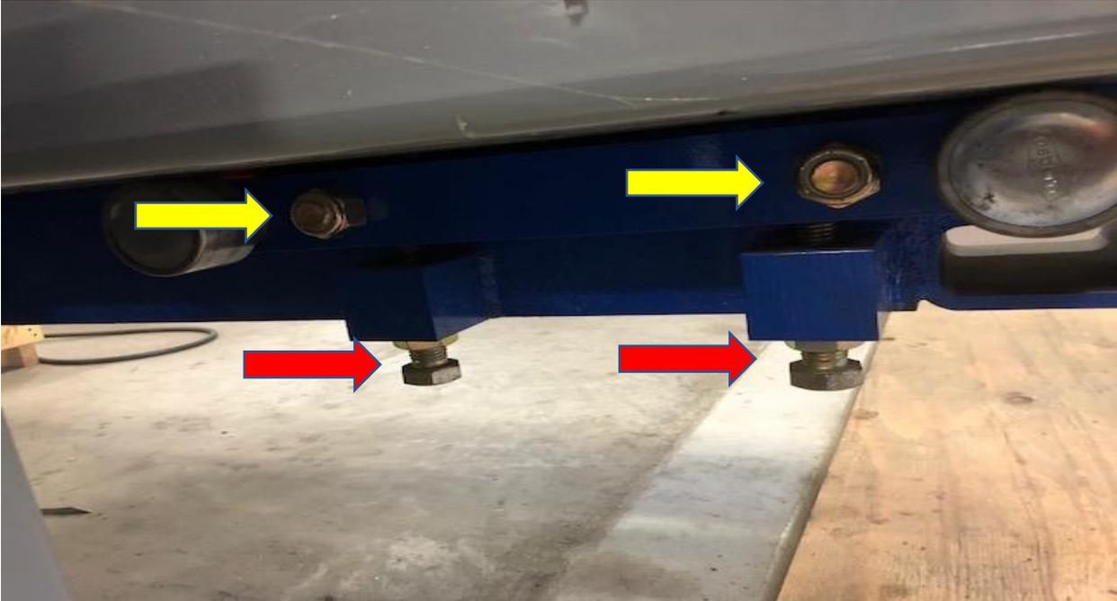
Location of Bogie Block Bolts and adjustment bolts and Jam Nuts.
